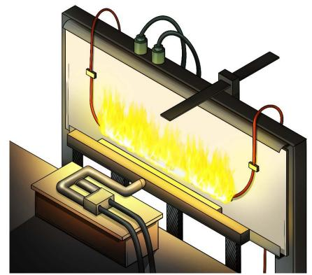
Resistance to fire with water spray - a new sample of cable is exposed to flame at 650°C for 15 minutes while passing a current at its rated voltage and then the spray is turned on to give exposure to both fire and water for a further 15 minutes.
