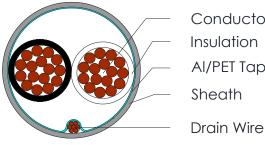
Conductor Insulation AI/PET Tape Sheath
